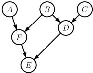
Write a sketch of a C program that uses Pthreads to execute the above six functions in a way that is maximally parallel, but adheres to the above dependency graph. Give a written explanation of how your code solves the problem. You can use any synchronization mechanism you want (join, condition variables, semeaphores, etc.).
